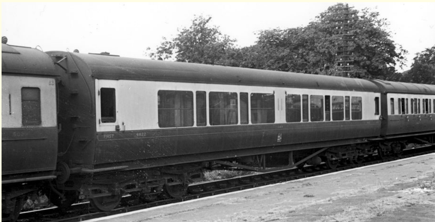
A GWR composite carriage, No.6622, built to Diagram E.151 in 1936. (Historical Model Railway Society)
