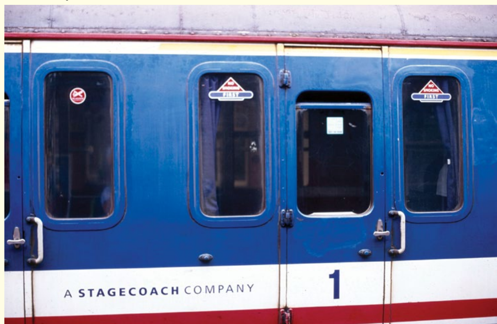
The BR Mk1 era as seen post-privatisation – first class compartments on a 4-VEP unit in Network SouthEast livery plus additional Stagecoach embellishments. The window stickers are pure BR. (Author)
