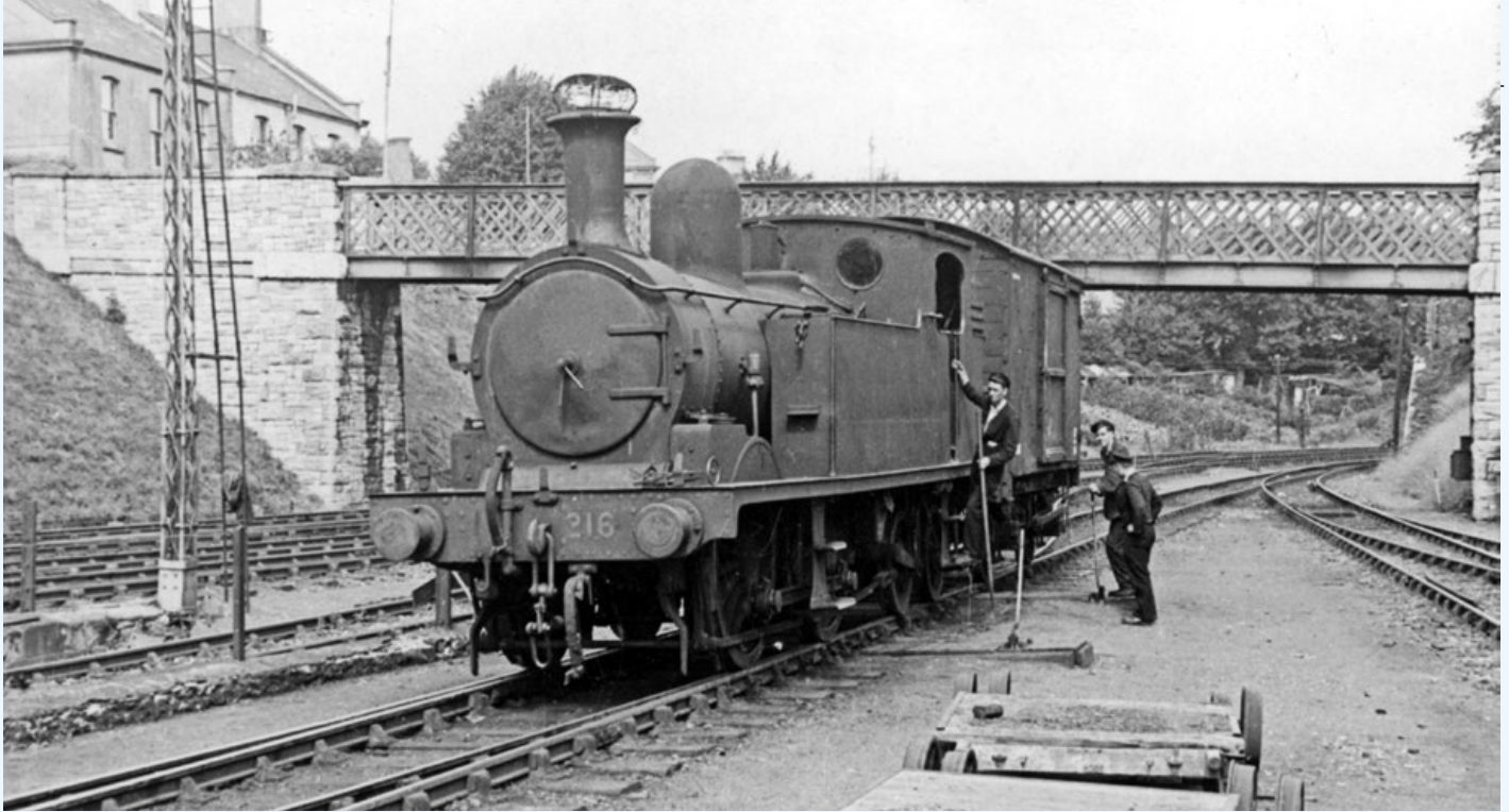
A spot of shunting is taking place at Devonport King's Road on 30th August 1945, with O2 0-4-4 tank No.216 (withdrawn in 1957) and attending goods shunters and pointmen. Note the characterful wire basket spark arrester, for shunting the timber yards at Oreston and probably of more imagined than real benefit. In the background the tracks disappear round the curve towards the GWR at Devonport Junction and North Road, whilst platelayers' trolleys rest on the ballast in the foreground. (H. C. Casserley)
