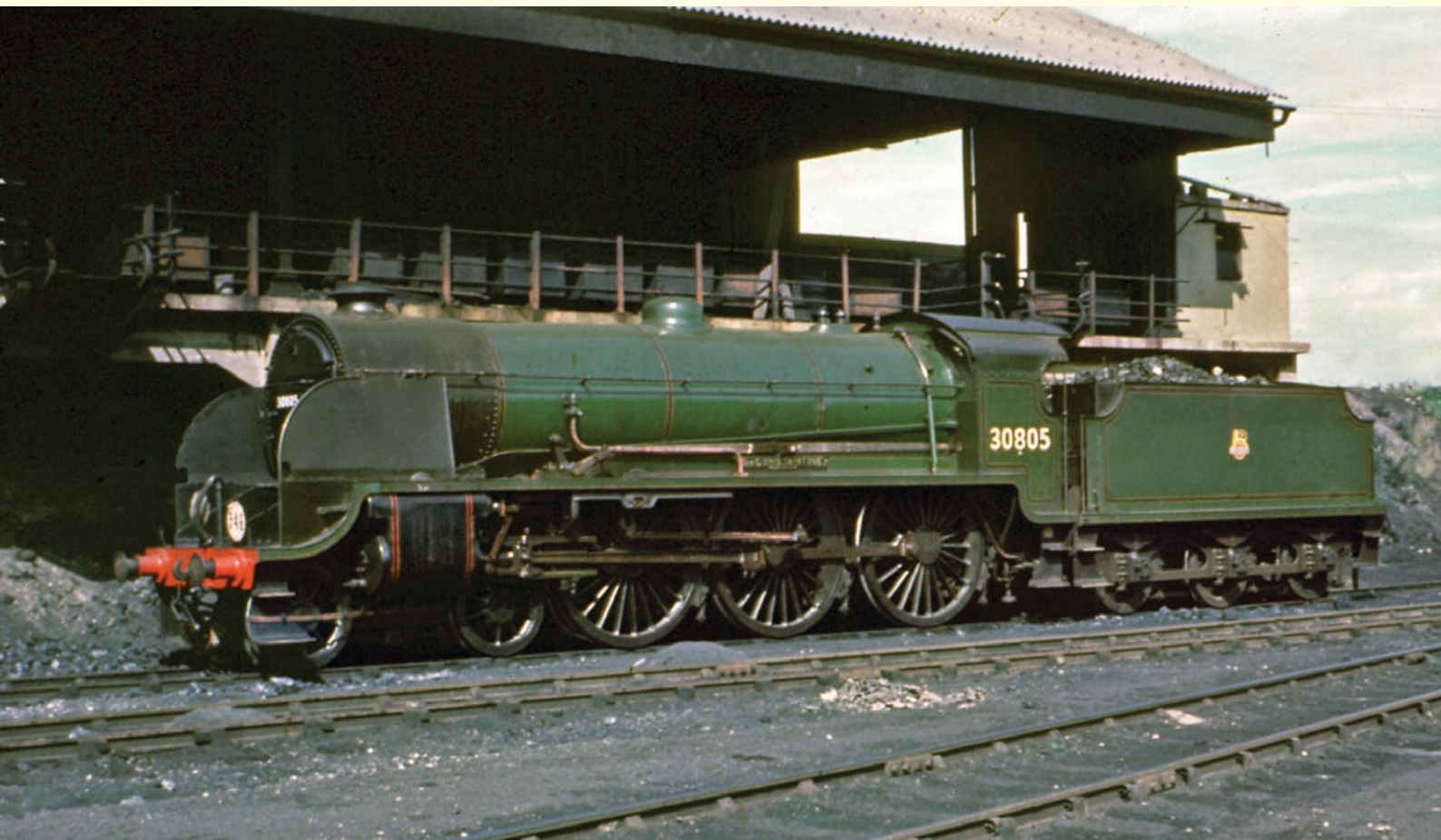
ABOVE: A very agreeable portrait of No.30805 Sir Constantine during an 'R and R' break in front of the coaling stage at Ashford shed on 23rd July 1953. Sir Harry was from the final order for N15s delivered from Eastleigh in 1926/7. They were intended for use on the Central Section of the SR (the Brighton lines) for which they were given smaller 3,500-gallon six-wheel tenders due to weight restrictions. (I. Davidson/Colour-Rail.com 308812)
