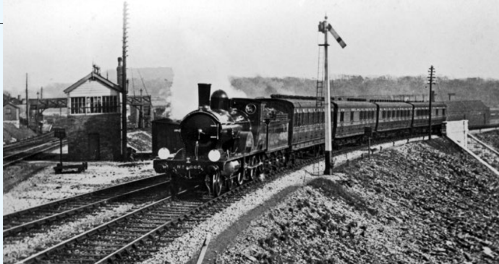
Gleaming Adams X6 4-4-0 No.660 in full LSWR livery and with striking stovepipe chimney proceeds round the south-to-west curve at Lipson Junction with a short express rake in about 1905, with the Great Western route to Exeter on the extreme left. The locomotive was to be withdrawn by the Southern Railway in October 1936. No X6s are preserved, sadly, but magnificent and very similar T3 No.563 was part of the National Collection until regrettably it was recently given away. (H. C. Casserley Collection)
