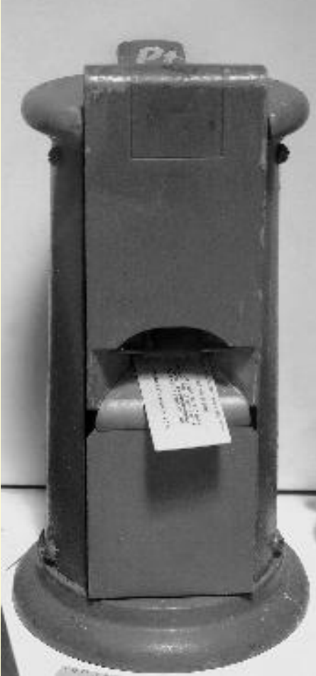
The ticket dating press was a long-lived part of the Edmondson process, using removable type and an inked ribbon to print the date. Alternative versions, which impressed the date unalterably, were also produced by Edmondson and other firms. (Author)
