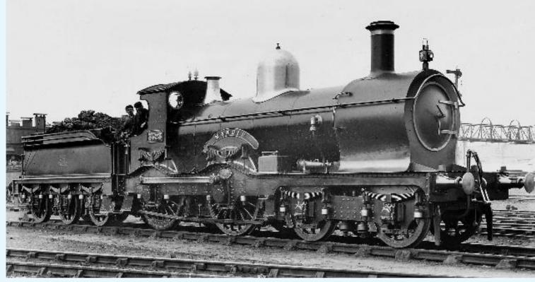
'Duke' No.3323 *Mendip* as originally built in 1899 with round-top boiler: what Hamilton Ellis described as the 'Olde English' style. It received a Belpaire boiler in 1907, reverted to a round-top boiler in 1910 (the only one to do so) and gained another Belpaire version in 1912. It was withdrawn as No.3288 in 1936. (Pendragon Collection)
