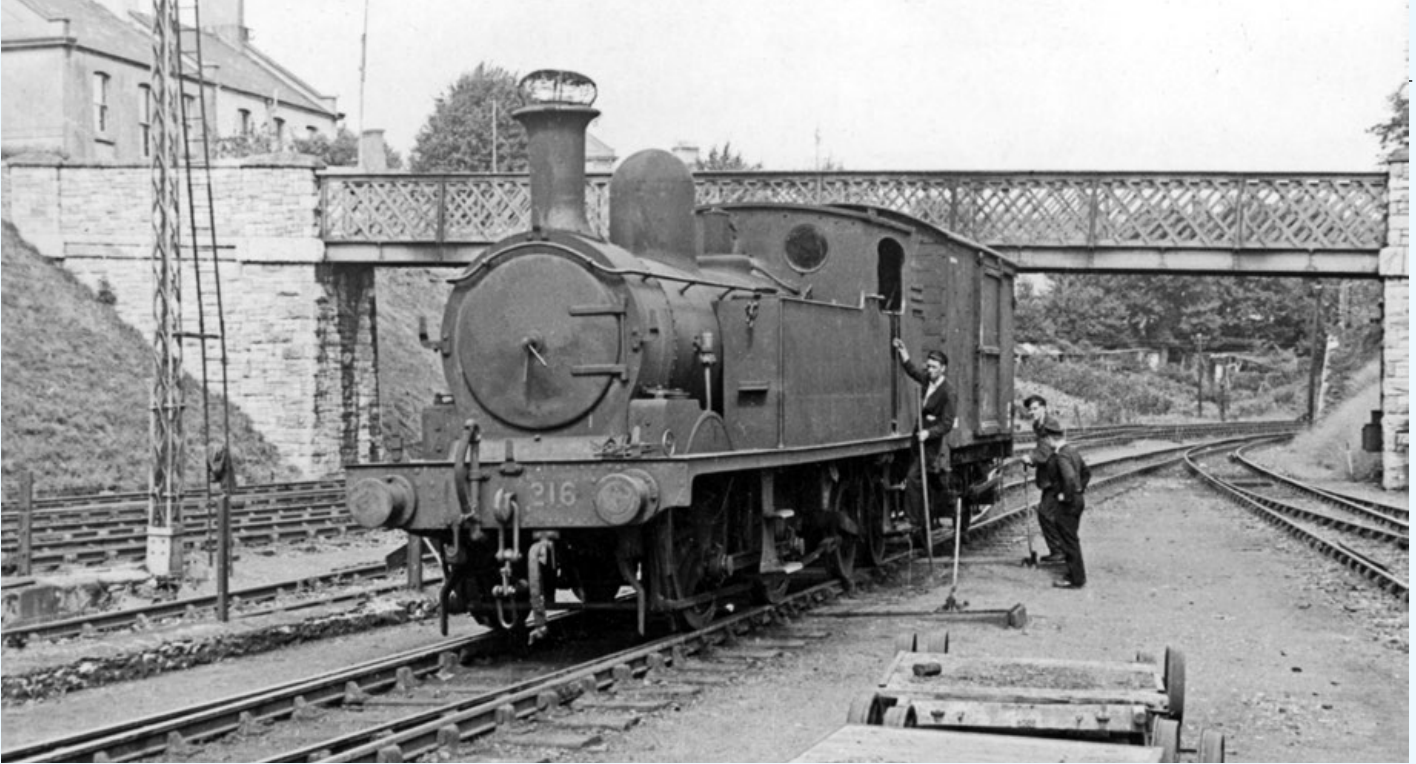
A spot of shunting is taking place at Devonport King's Road on 30th August 1945, with O2 0-4-4 tank No.216 (withdrawn in 1957) and attending goods shunters and pointsmen. Note the characterful wire basket spark arrester, for shunting the timber yards at Oreston and probably of more imagined than real benefit. In the background the tracks disappear round the curve towards the GWR at Devonport Junction and North Road, whilst platelayers' trolleys rest on the ballast in the foreground. (H. C. Casserley)
